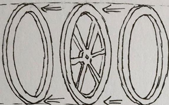
Assemble the two wheels, with the spacers in the middle.
